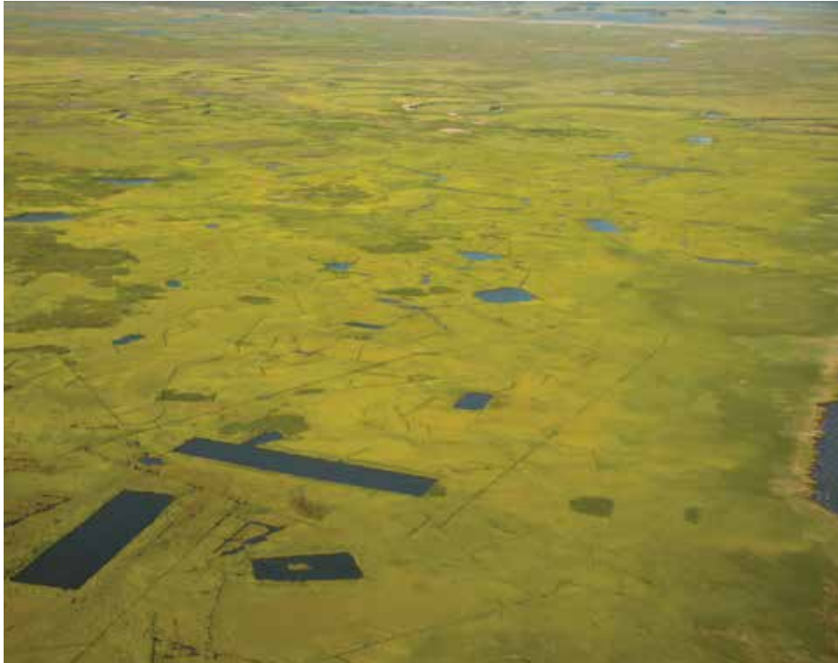
Throughout vast areas of the Atlantic Coast, tidal marshes have been ditched and modified for mosquito control. This practice alters the hydrology of the marsh and may be contributing to black rail declines. Photo by Bart Paxton
